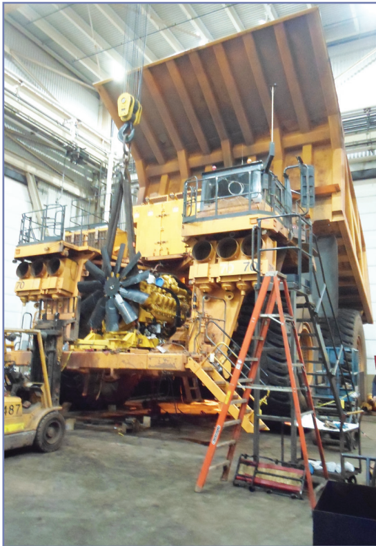
A repower in progress
